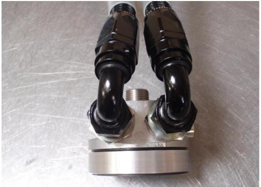
3. Place the spacer plate assembly were the oil filter screws on, tighten TO 30-35LBFT in position shown below making sure there is clearance all around and then replace oil filter.
